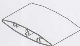
The Eclipse system is comprised of aluminium and 316 marine grade stainless components with a high level of corrosion resistance.
